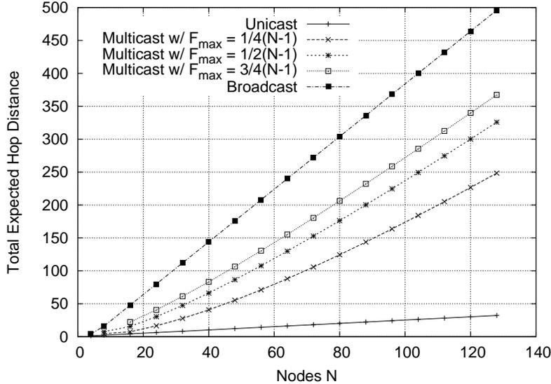
Fig. 1. Total expected hop distance  $E[H]$  of shortest path routing bidirectional WDM ring with  $\Lambda = 4$  vs. number of nodes  $N$  for unicast, broadcast, and multicast traffic with different maximum multicast fanout  $F_{\max} \in \{1/4(N-1), 1/2(N-1), 3/4(N-1)\}$ .
