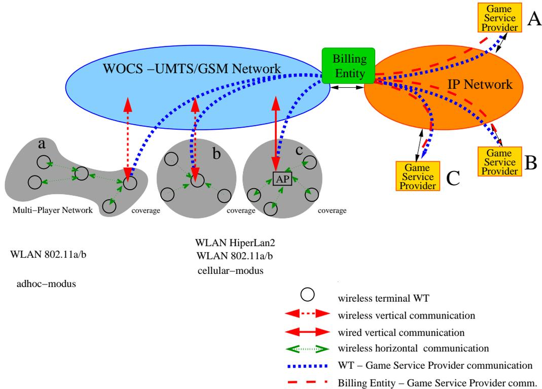
Figure 1: Vertical and horizontal communication structure for a multi-player gaming session with billing
