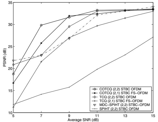
Fig. 4. Image PSNR as a function of channel SNR for COTCQ and TCQ with (2,1) STBC FS-OFDM and with (2,2) STBC OFDM, compared with MDC-SPIHT and SPIHT with (2,2) STBC OFDM for Lenna image at 0.5bpp.
