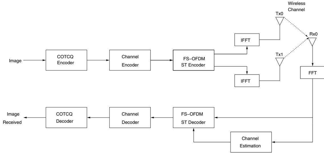
Fig. 1. System structure for image transmission over FS-OFDM system using (2,1) STBC
