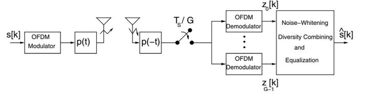
Fig. 3. Block diagram of FS-OFDM system.
