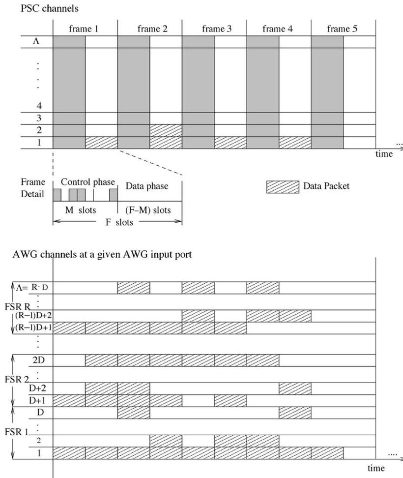
Fig. 4. AWG-PSC mode timing structure: The pretransmission coordination is conducted over a control wavelength channel (one of the  $\Lambda$  wavelength channels) on the PSC during the control phase. During the data phase, data packets are transmitted over the  $\Lambda$  PSC wavelength channels. The  $\Lambda$  wavelength channels at each of the  $D$  AWG ports are used for data packet transmission all the time.
