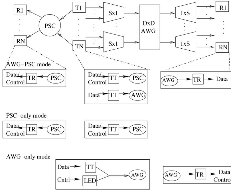
Fig. 3. Detailed node architecture with transmitter and receiver connections to the AWG and to the PSC for the three different modes of operation. A given node’s transmitter and receiver are colocated, e.g., T1 and R1 are at the same location. The AWG and PSC are arranged in parallel; the network is “unfolded” here for illustration.
