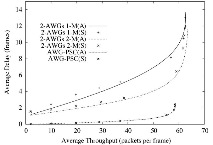
Fig. 13. Throughput-delay performance comparison for three networks:  $D$ -buffered AWG||AWG with one control,  $D$ -buffered AWG||AWG with two controls, and AWG||PSC.
