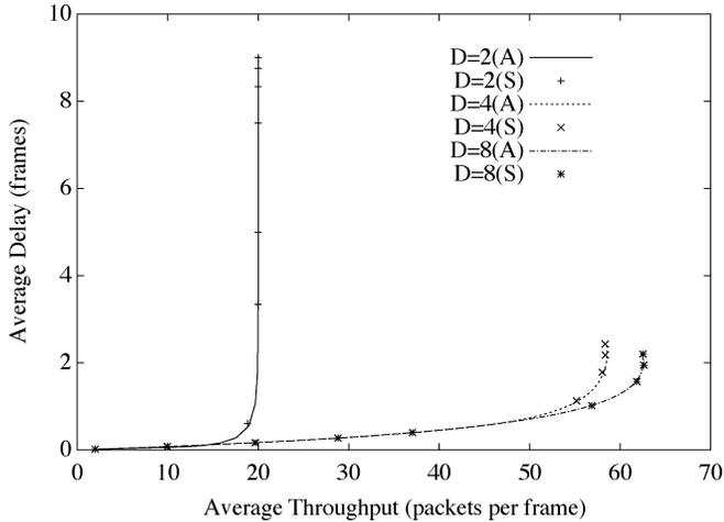
Fig. 8. Throughput-delay performance for AWG-PSC mode for AWG degree  $D = 2, 4,$  and  $8.$  ( $R = 2$  fixed).
