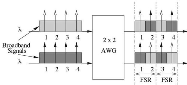
Fig. 1. Periodic wavelength routing of an AWG with  $D = 2$  input and output ports when  $R = 2$  FSRs are used. Each FSR provides one wavelength channel between an I/O port pair. A total of  $D \cdot D \cdot R = D \cdot \Lambda = 2 \cdot 4$  wavelength channels connect the input ports to the output ports.
