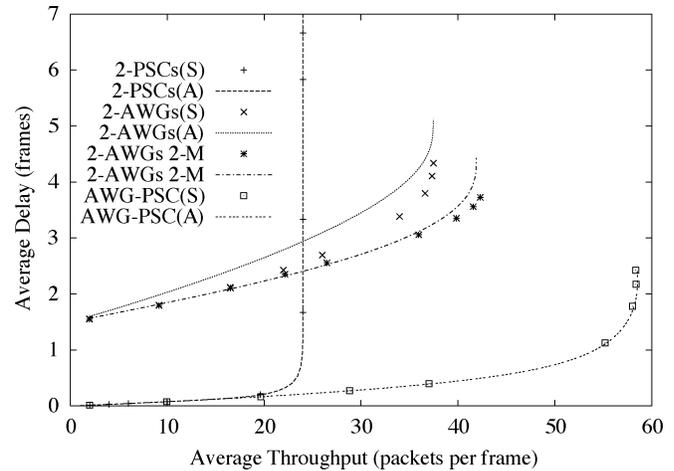
Fig. 12. Throughput-delay performance comparison for three networks: PSC||PSC, AWG||AWG, and AWG||PSC.
