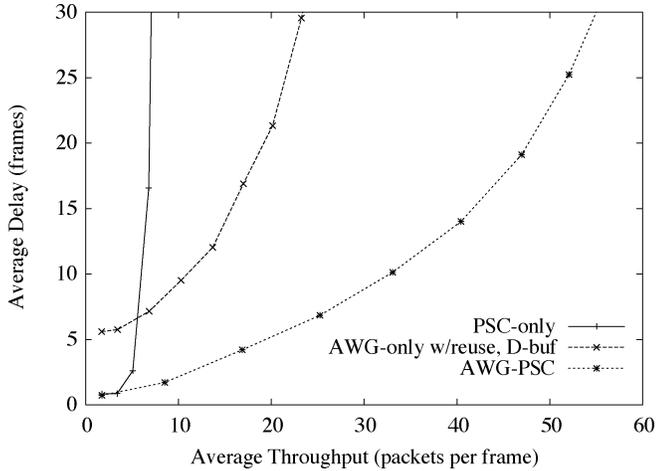
Fig. 14. Throughput-delay performance of AWG||PSC network for three modes of operation for self-similar traffic and large node buffers.
