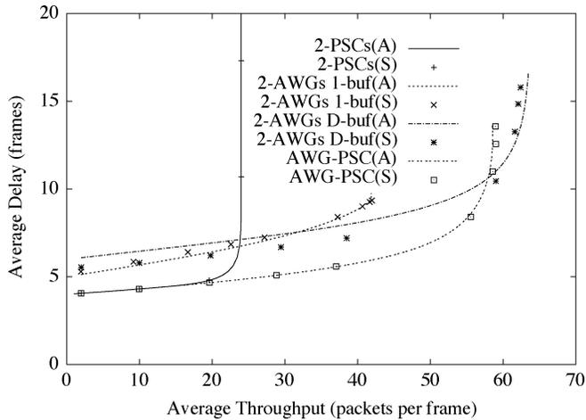
Fig. 16. Throughput-delay performance comparison for two-device networks for a propagation delay of  $\tau = 4$  frames ( $N = 200$  fixed).
