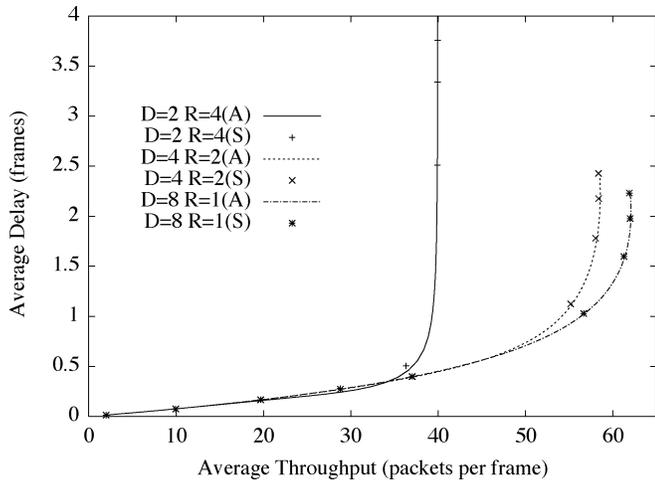
Fig. 10. Throughput-delay performance for AWG-PSC mode for fixed tuning range  $\Lambda = R \cdot D = 8$  wavelengths.
