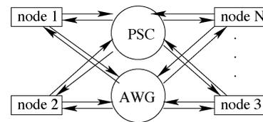
Fig. 2. Network architecture with parallel fiber connections from each of the  $N$  nodes to the AWG and to the PSC.
