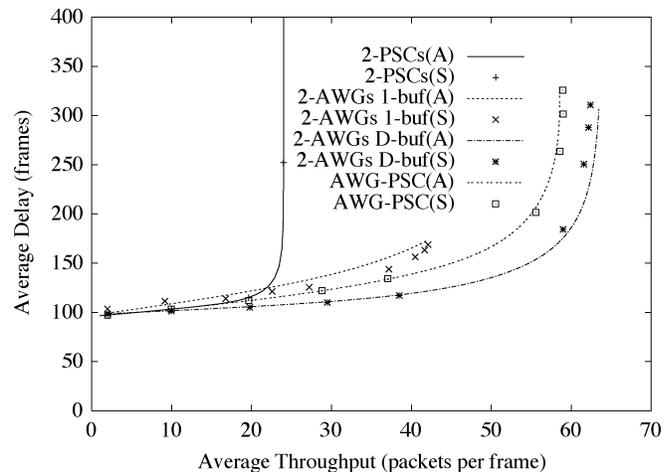
Fig. 18. Throughput-delay performance comparison for two-device networks for a propagation delay of  $\tau = 96$  frames ( $N = 200$  fixed).
