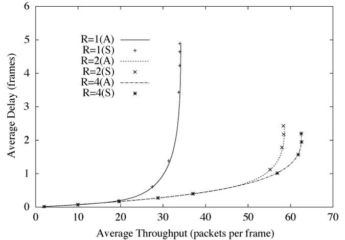
Fig. 9. Throughput-delay performance for AWG-PSC mode for  $R = 1, 2,$  and  $4$  used FSRs. ( $D = 4,$  fixed).
