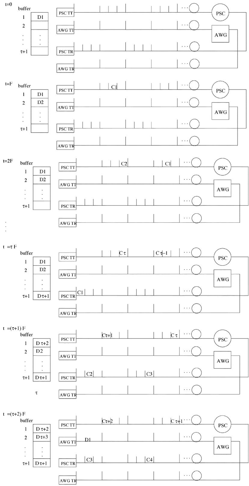
Fig. 15. Illustration of time-sequenced buffering.
