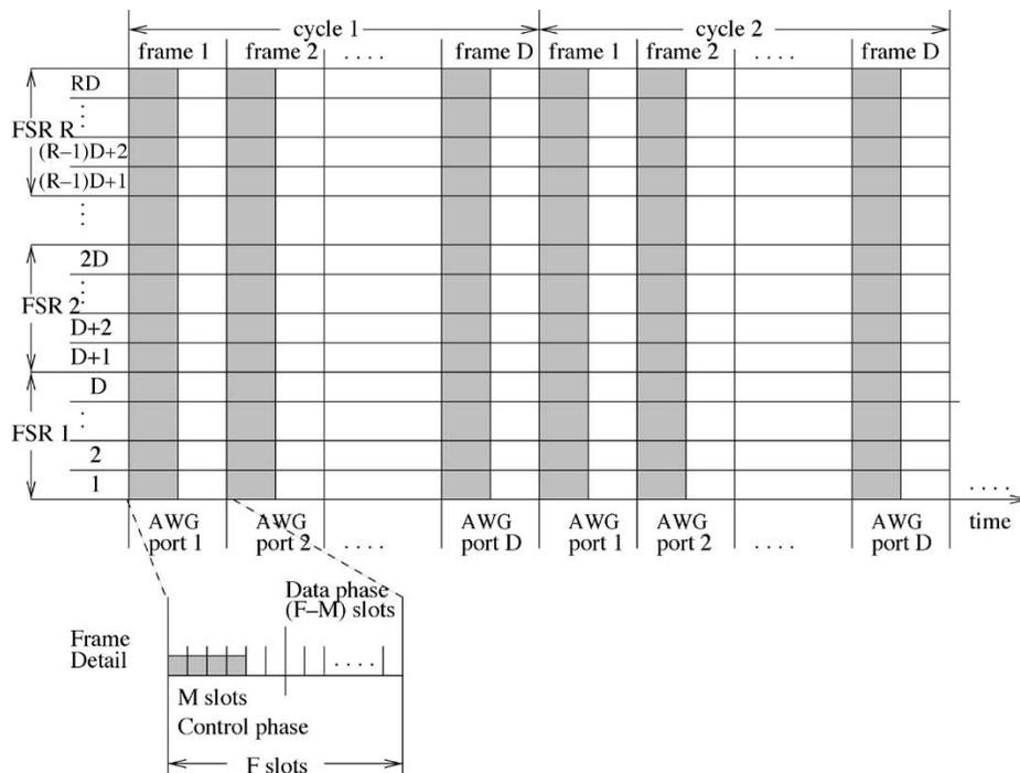
Fig. 6. AWG-only mode timing structure.
