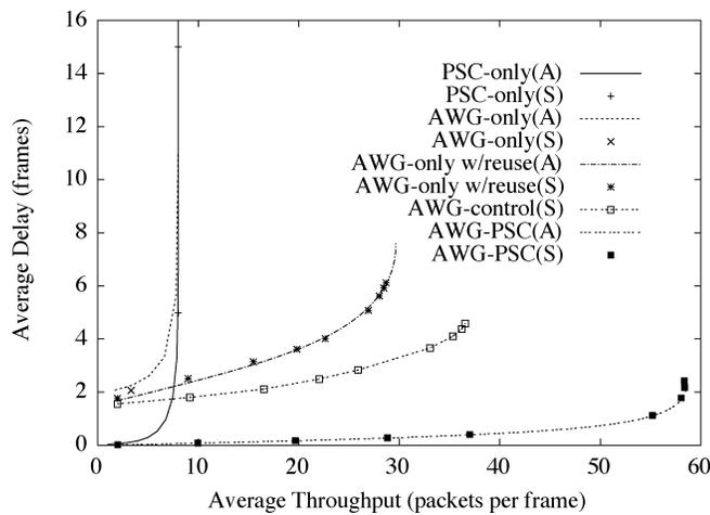
Fig. 11. Throughput-delay performance of AWG||PSC network for different modes of operation.
