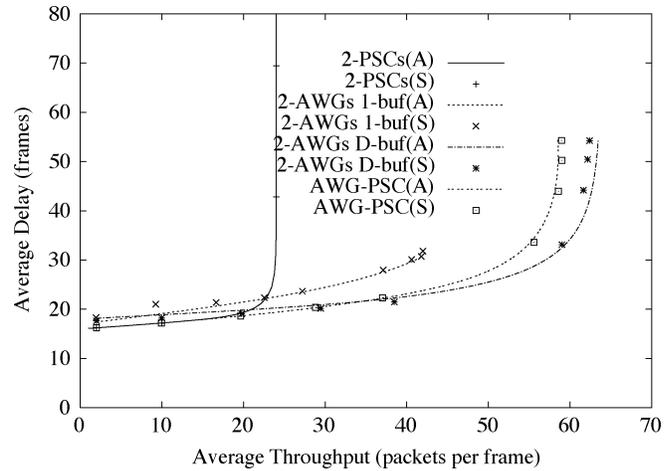
Fig. 17. Throughput-delay performance comparison for two-device networks for a propagation delay of  $\tau = 16$  frames ( $N = 200$  fixed).
