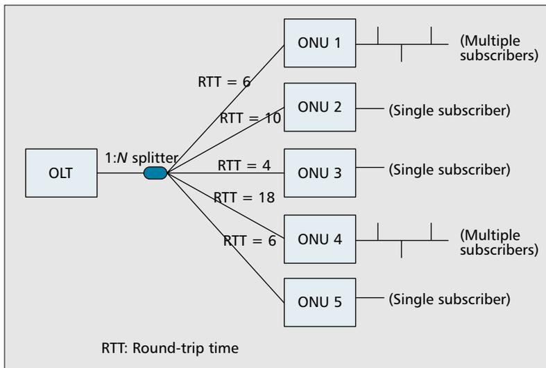
**FIGURE 1.** Network architecture of an EPON with one optical line terminal (OLT) and  $N = 5$  optical network units (ONUs), each with a different round-trip time (RTT).
