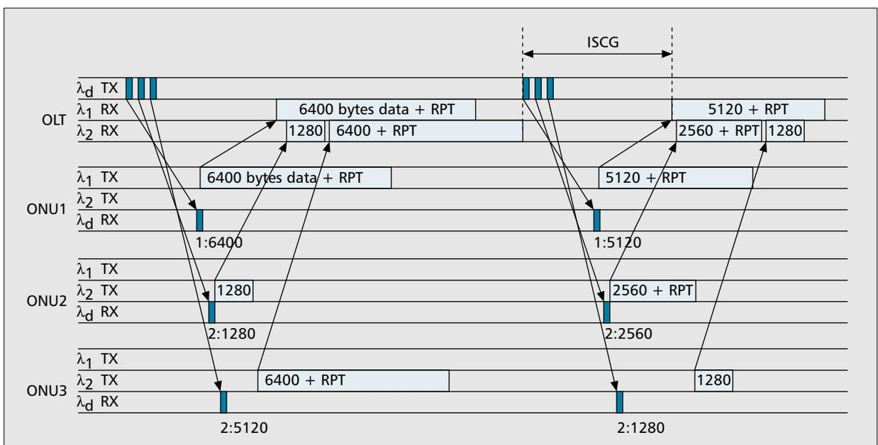
**FIGURE 4.** Illustration of the offline scheduler, which introduces the ISCG between successive cycles.
