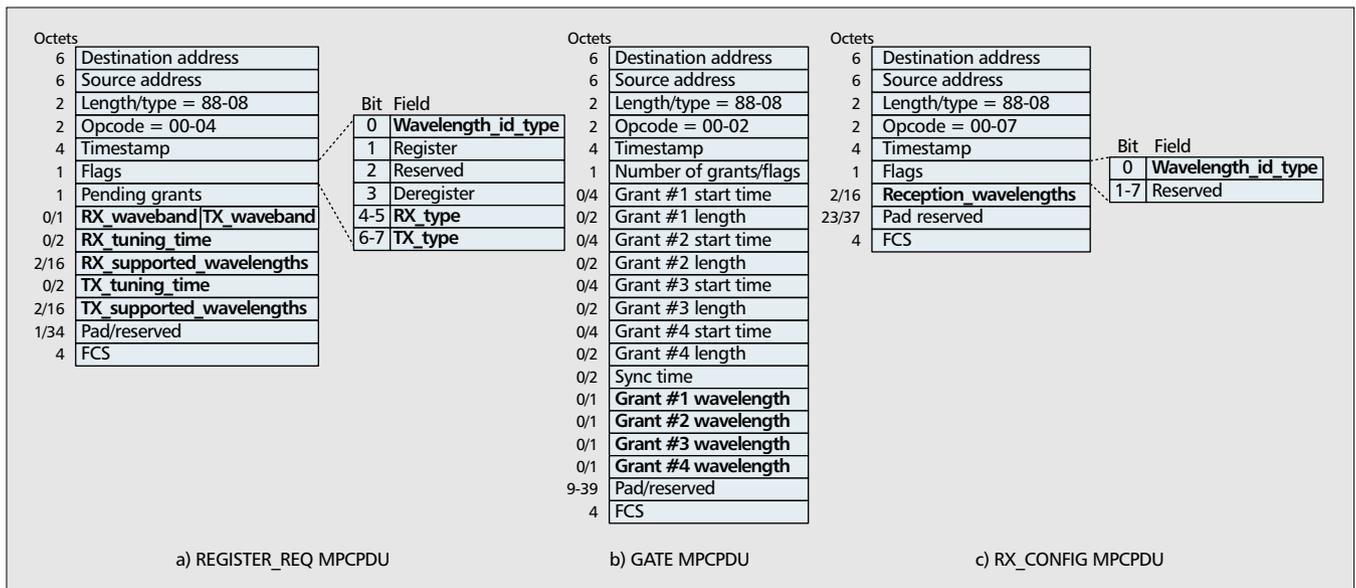
**FIGURE 2.** WDM extensions to MPCP protocol data units (PDUs): a) REGISTER\_REQ; b) GATE; c) the proposed RX\_CONFIG (extensions are shown bold).
