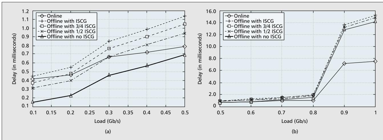
FIGURE 5. Comparison of packet delay with online and offline scheduling on a five-wavelength EPON as a function of load: a) lower load; b) higher load.
