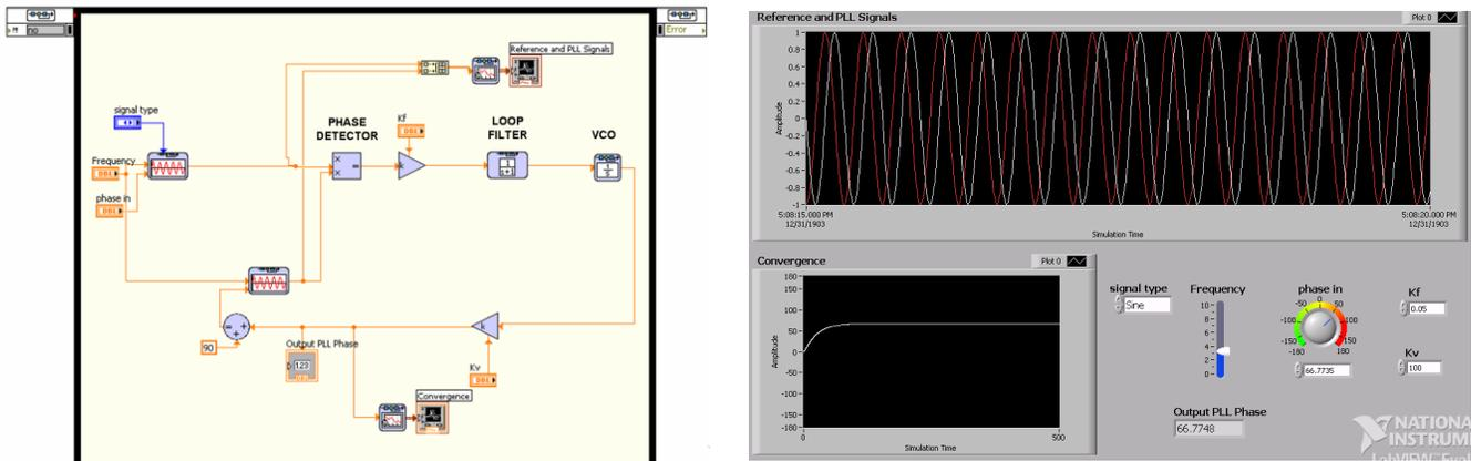
Figure 1. Block diagram and Front panel for the design of a Phase Locked Loop (PLL).
