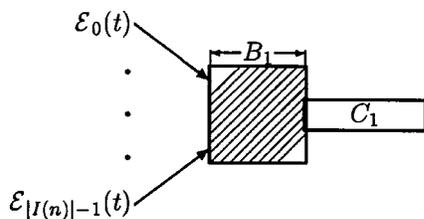
Fig. 7. Traffic of connection  $j$  is characterized by the regulator function  $\mathcal{E}_j(t)$  and fed directly, i.e., unsmoothed, into a buffered multiplexer.
