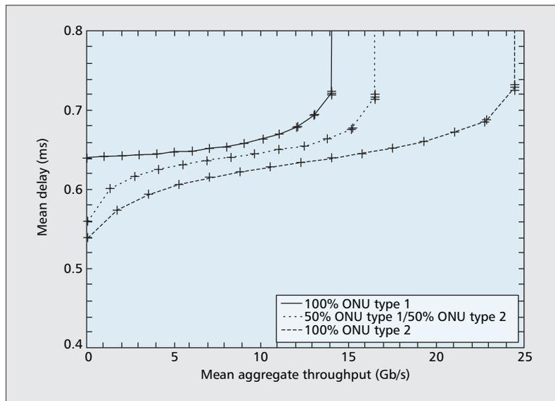
■ **Figure 6.** Mean delay vs. mean aggregate throughput of STARGATE for limited service.
