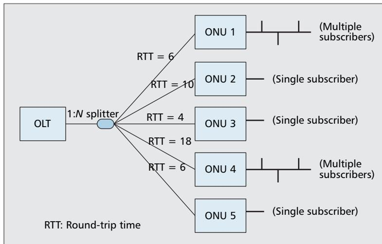
■ **Figure 1.** EPON architecture with one optical line terminal (OLT) and  $N = 5$  optical network units (ONUs), each with a different round-trip time.
