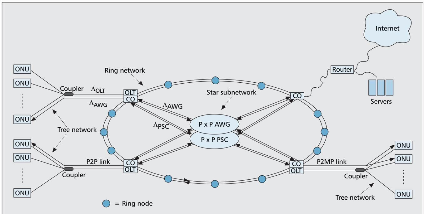
■ Figure 2. STARGATE network architecture comprising  $P = 4$  central offices (COs) and  $N_r = 12$  RPR ring nodes.
