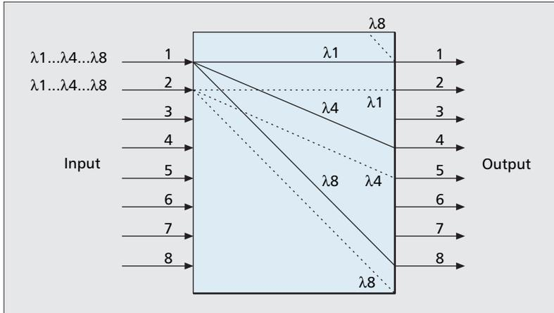
■ **Figure 4.** Wavelength routing of an  $8 \times 8$  arrayed waveguide grating.
