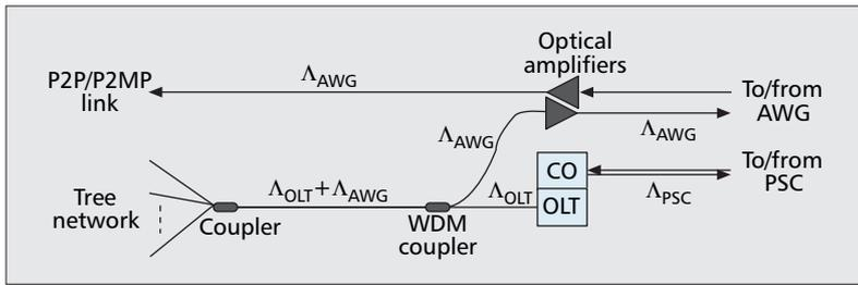
■ **Figure 3.** Optical bypassing of optical line terminal and central office.
