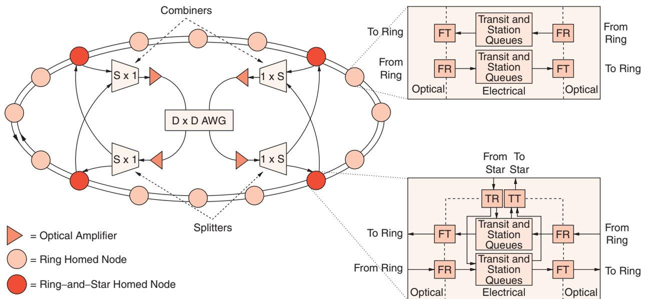
**Fig. 4 WDM on star subnetwork: a subset  $P = 4$  of  $N = 12$  RPR nodes are interconnected by an AWG-based single-hop star WDM subnetwork**
