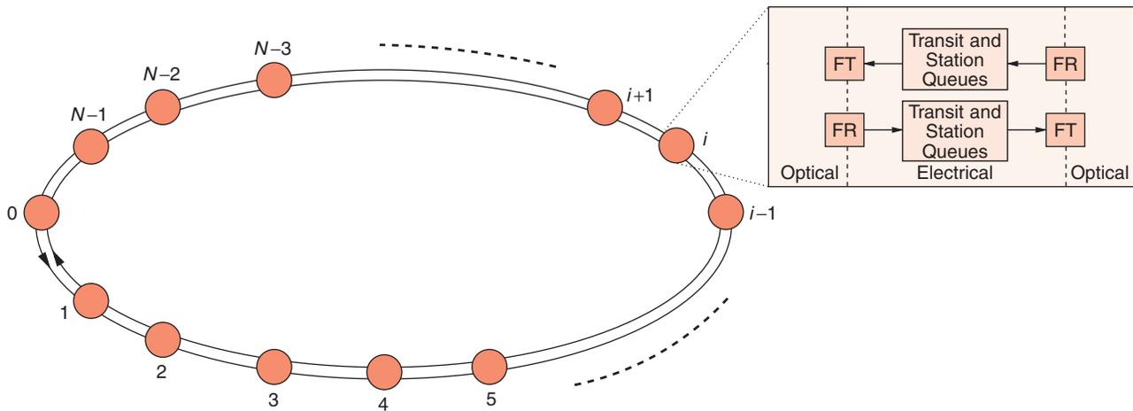
**Fig. 1** Illustration of a resilient packet ring (RPR) network interconnecting  $N$  nodes and the node architecture
