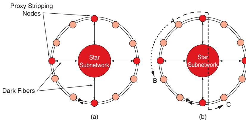
**Fig. 3 Proxy stripping technique: (a) architecture: RPR with  $N = 12$  nodes, where  $P = 4$  nodes are interconnected by a dark-fiber single-hop star subnetwork; (b) operation: packets are sent on the shortest path and stripped by the destination**
