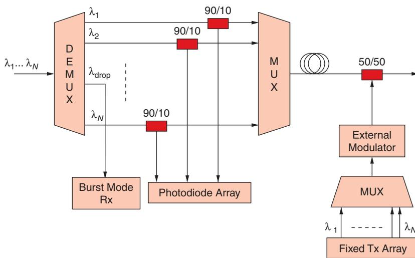
**Fig. 2 Example node architecture of a WDM ring network: the signals on drop wavelength  $\lambda_{\text{drop}}$  are converted to the electrical domain and the signals on the other wavelengths stay in the optical domain**
