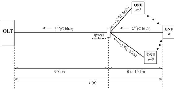
Fig. 1. Illustration of upstream transmission direction from distributed ONUs  $o, o = 1, 2, \dots, O$ , to a central OLT in the PON structure. The  $O$  ONUs share a single wavelength channel with bit rate  $C$  bit/s for their upstream transmissions and have one-way propagation delay  $\tau(o)$  to the OLT.
