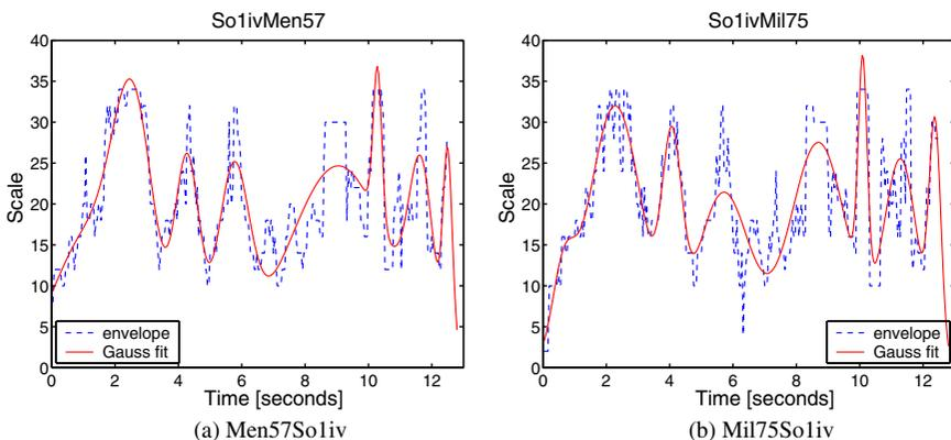
Fig. 3. Numerical wavelet envelope function and corresponding analytical Gaussian fit.
