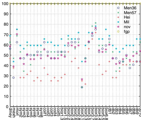
Fig. 7. Percentages of correctly identified pieces with probabilistic radial network for different wavelets. The morlet and bior3.9 wavelet achieve good generalization.
