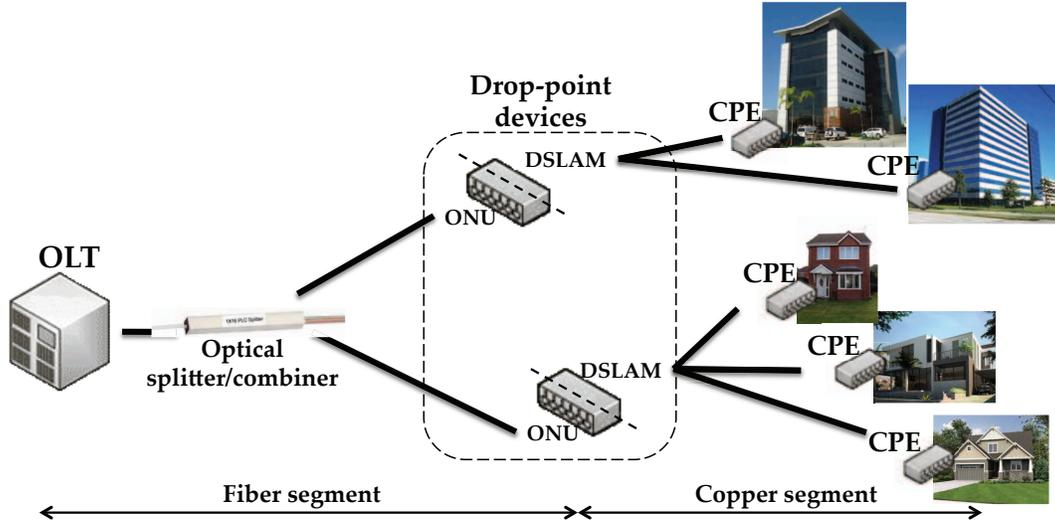
Fig. 2. Hybrid PON/xDSL access network. The device that bridges the fiber and copper portions of the network is a combined ONU and DSL access multiplexer (DSLAM) called a drop-point device.
