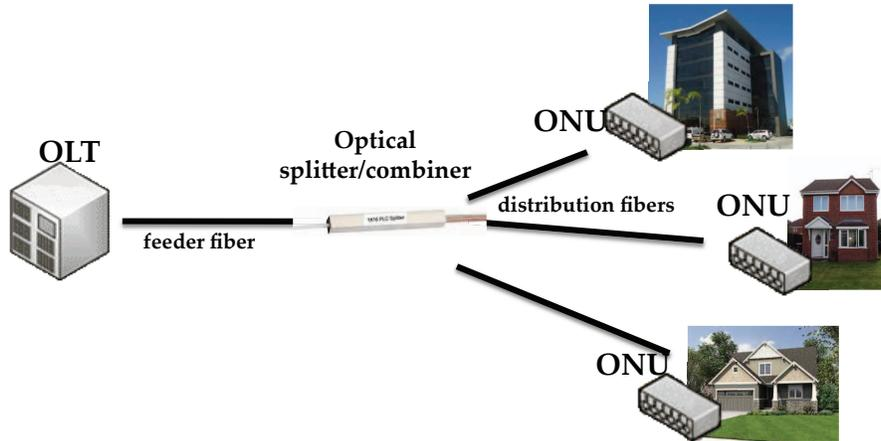
Fig. 1. A passive optical network (PON). An Optical Line Terminal (OLT) connects to multiple Optical Network Units (ONUs) via feeder fiber optic cable that is in close proximity to a set of subscribers and several distribution fiber optic cables. The optical transmission power on the feeder fiber is split for transmission on several distribution fibers that are connected to individual ONUs.
