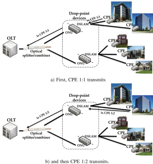
Fig. 4. In the segregated strategy, the DSL CPEs attached to the same drop-point device transmit one at a time.
