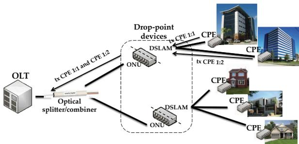
Fig. 5. In the multiplexed strategy, the DSL CPEs attached to the same drop-point device transmit at the same time. Their data subsequently appears multiplexed on the PON segment.
