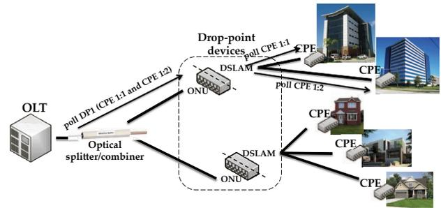
Fig. 3. The OLT polls a drop-point device (DP1) to grant upstream transmission access. Included in the polling message are polling messages for the DSL CPEs attached to DP1, CPE 1:1 and CPE 1:2. These CPE polling messages indicate when and for how long each DSL CPE should transmit.
