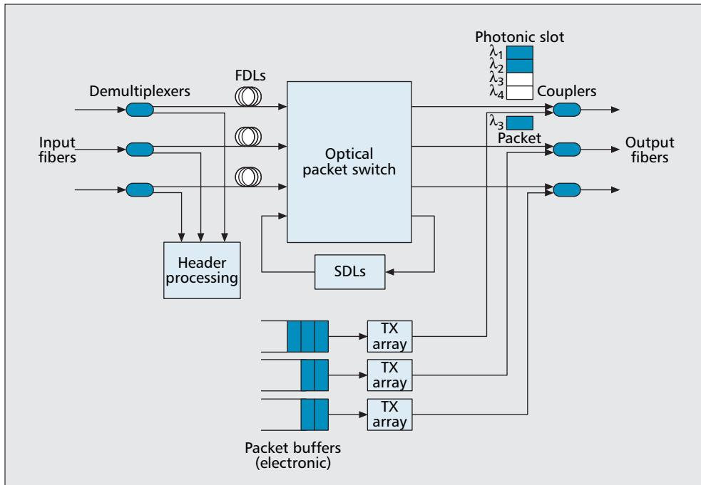
■ Figure 2. PSR node with multiple input/output ports [13].
