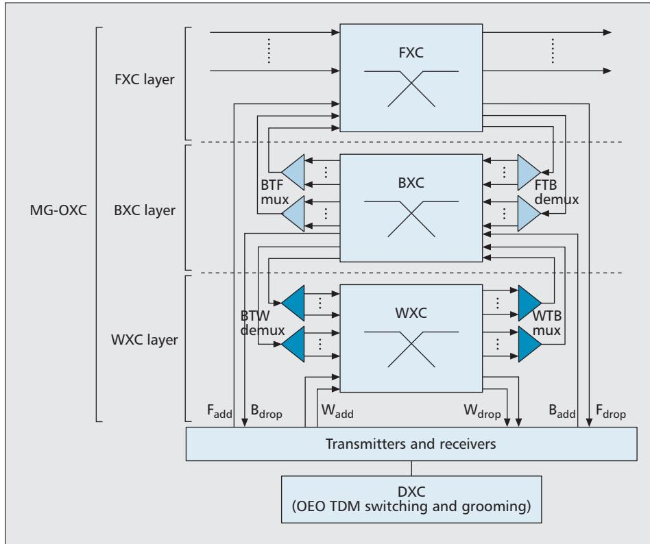
■ Figure 1. Multigranularity photonic cross-connect consisting of a three-layer multigranularity optical cross-connect (MG-OXC) and a digital cross-connect (DXC) [3].
