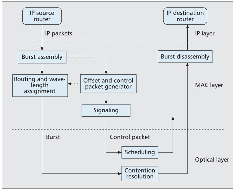
■ Figure 4. Block diagram of OBS networks consisting of IP, MAC, and optical layers [22].
