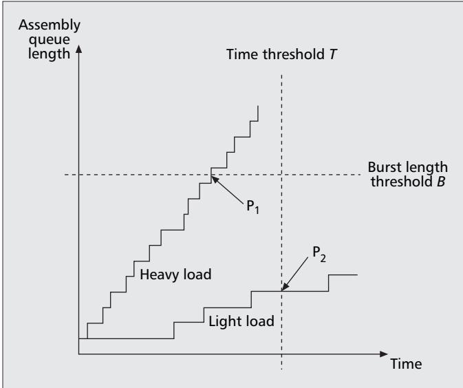
■ Figure 3. Burst length and time thresholds for burst assembly algorithms [19].
