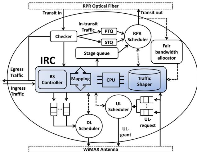
Fig. 8. Optical-wireless interface between RPR and WiMAX networks
