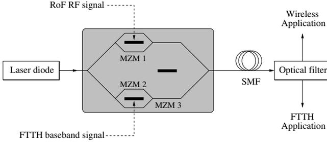
**Fig. 2.** Simultaneous modulation and transmission of FTTH baseband signal and RoF RF signal using an external integrated modulator consisting of three Mach-Zehnder modulators (MZMs) [12]
