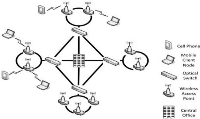
**Fig. 5.** Optical hybrid star-ring network integrated with WiFi-based wireless access points [21]
