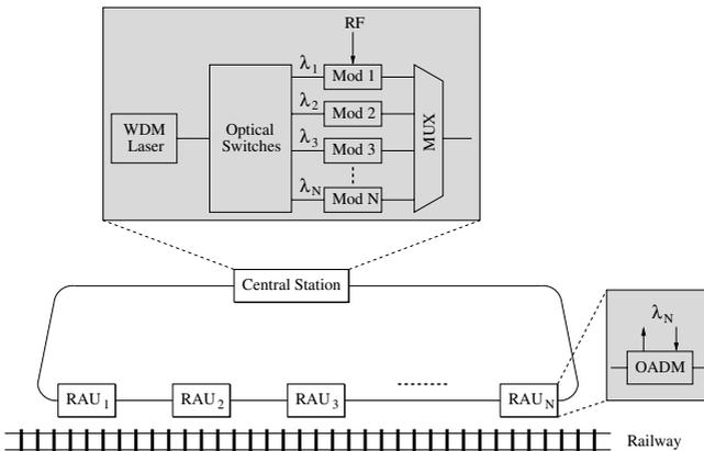
**Fig. 3.** Moving cell-based RoF network architecture for train passengers [19]
