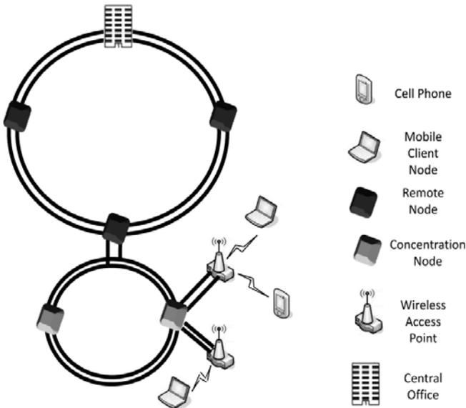
**Fig. 4.** Optical interconnected bidirectional fiber rings integrated with WiFi-based wireless access points [20]
