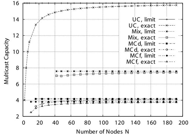
Fig. 2. Multicast capacity of bidirectional ring with two copy transmission: Comparison of exact  $C_M^{b,N}$  with  $\lim_{N \rightarrow \infty} C_M^{b,N}$ ;  $\Lambda_b = 2$ , fixed
