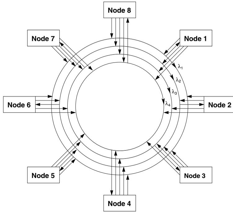
Fig. 1. Unidirectional WDM ring network connecting  $N = 8$  nodes with  $\Lambda = 4$  wavelength channels; each wavelength channel homes  $\eta_u = N/\Lambda = 2$  nodes. In the corresponding bidirectional ring there are  $\Lambda_b = \Lambda/2 = 2$  wavelength channels operated in each direction, with each wavelength channel homing  $\eta_b = N/\Lambda_b = 4$  nodes.
