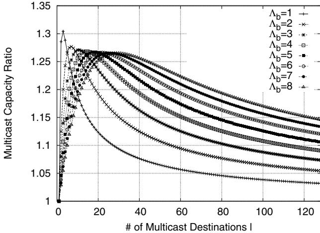
Fig. 5. Capacity ratio (gain) with two copy transmission over one copy transmission in bidirectional ring network  $\lim_{N \rightarrow \infty} C_M^{b,N}(l)/C_M^{u,N}(l)$  for fixed fanout  $F = l$  as a function of number of wavelengths  $\Lambda_b$  and destinations  $l$ .
