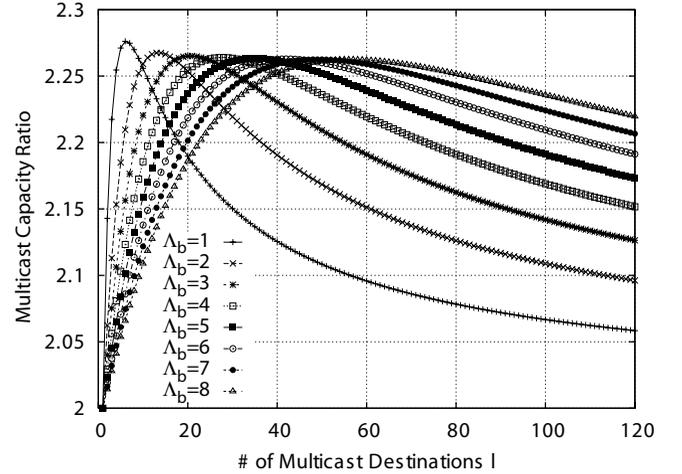
Fig. 4. Multicast capacity ratio  $\lim_{N \rightarrow \infty} C_M^{b,N}(l)/C_M^{u,N}(l)$  (with two copy transmission in bidirectional ring) for fixed fanout  $F = l$  as a function of number of wavelengths  $\Lambda_b$  and destinations  $l$ .
