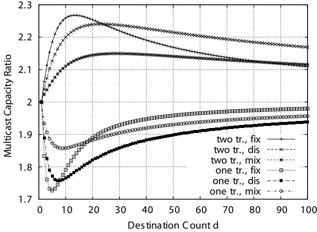
Fig. 3. Multicast capacity ratios  $\lim_{N \rightarrow \infty} C_M^{b,N}/C_M^{u,N}$  (with two copy transmission in bidir. ring) and  $\lim_{N \rightarrow \infty} C_M^{b1c,N}/C_M^{u,N}$  (with one copy transmission in bidir. ring) as a function of maximum destination count  $d$ ;  $\Lambda_b = 2$ , fixed.
