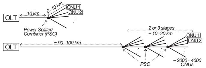
Fig. 1. Differences between PON (top) and LR-PON (bottom) topologies.
