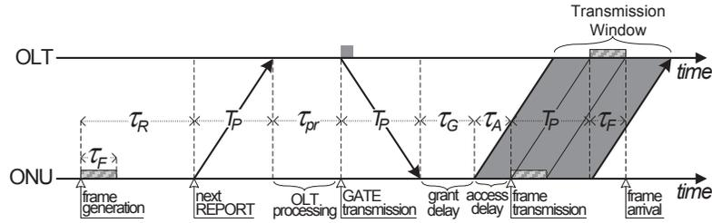
Fig. 2. Frame delay components in polling.
