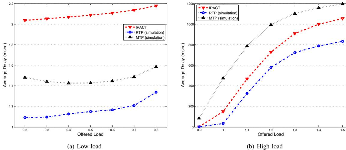
Fig. 6. Delay performance of DBA methods with limited service when  $\tau = 500\mu\text{s}$  (100km)
