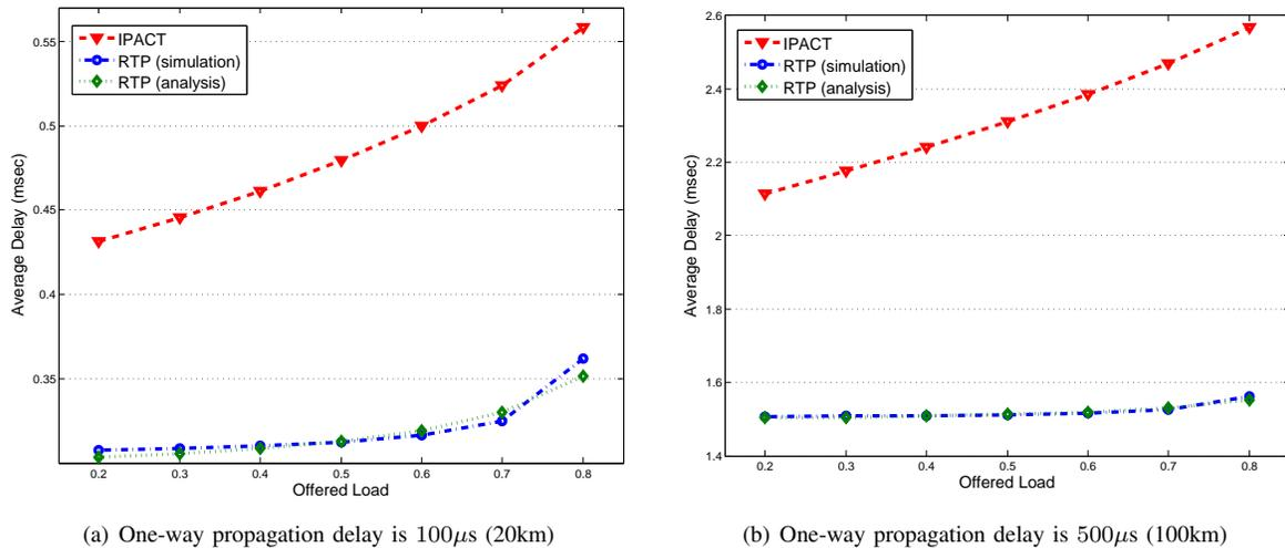
Fig. 3. Delay comparison for conventional polling and ERT-P with gated service
