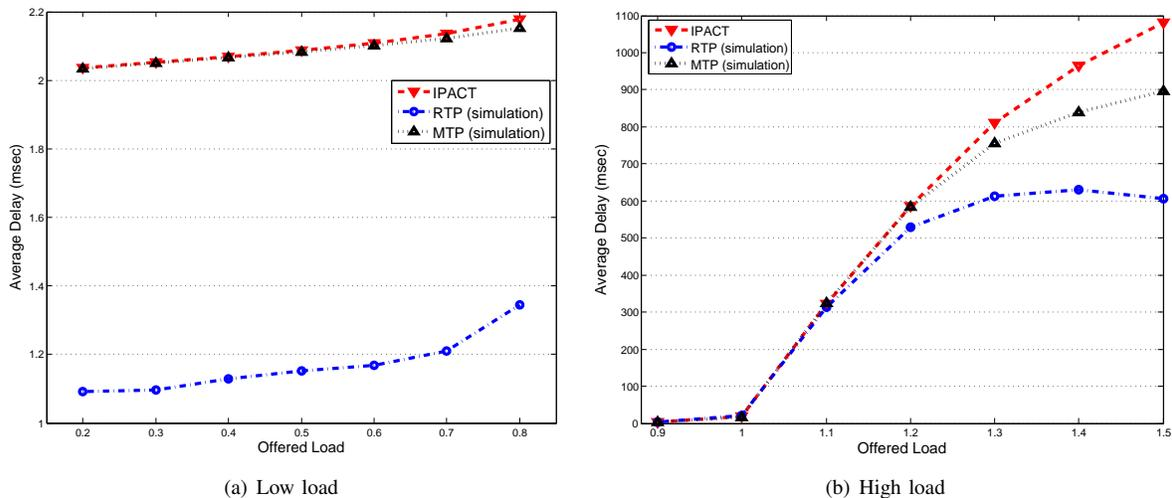
Fig. 5. Delay performance of DBA methods with gated service when  $\tau = 500\mu\text{s}$  (100km)
