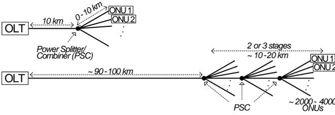
Fig. 1. Differences between PON (top) and LR-PON (bottom) topologies.
