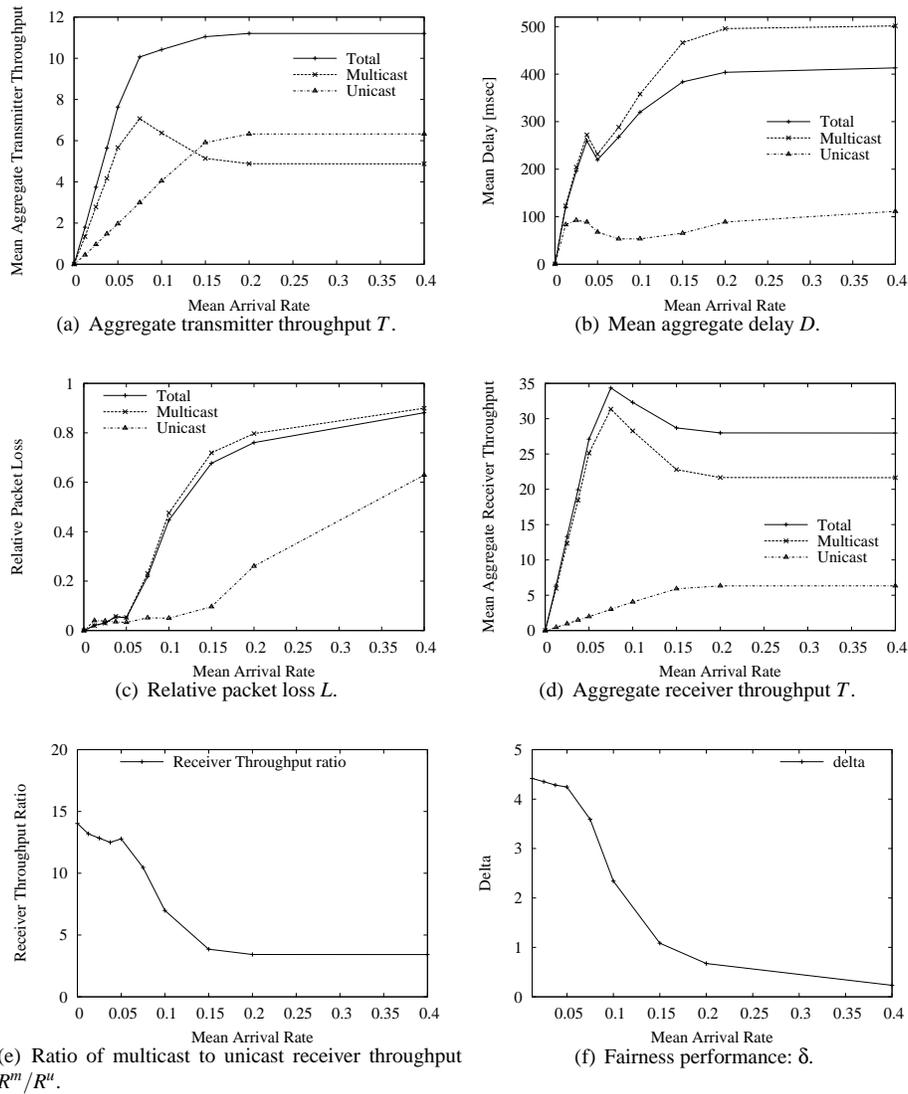
Fig. 6. Performance for  $(\Lambda + \Lambda)$ VOQ architecture with channel-priority policy with  $w = 0$ .
