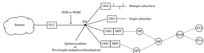
Fig. 1. FiWi network architecture based on single- or multi-stage TDM or WDM PON and multihop WMN (MPP: Mesh Portal Point, MP: Mesh Point, STA: Wireless Station).
