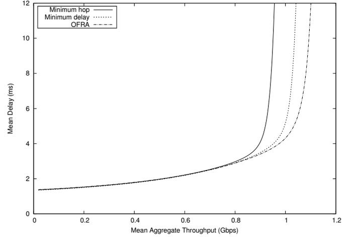
Fig. 3. Mean delay vs. mean aggregate throughput performance of different FiWi routing algorithms for a conventional wavelength-routing WDM PON of 20 km range and  $B = 1$ .
