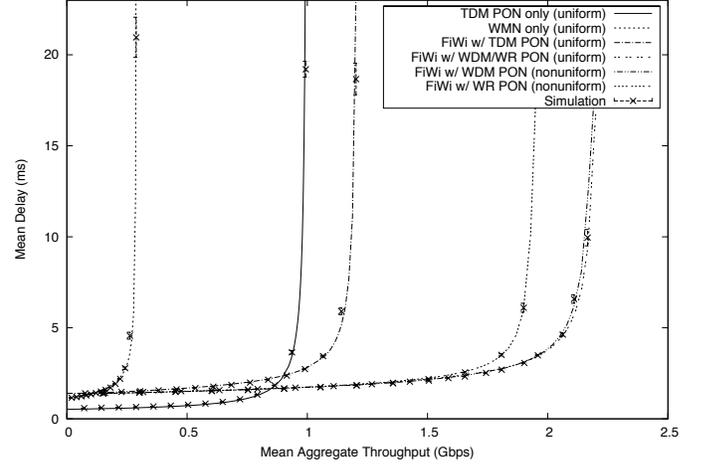
Fig. 2. Mean delay vs. mean aggregate throughput performance of different FiWi network architectures for uniform and nonuniform traffic (simulation results are shown with 95% confidence intervals).
