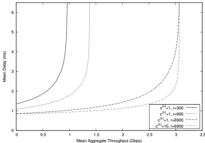
Fig. 5. Mean delay vs. mean aggregate throughput performance of next-generation FiWi access networks based on high-speed wavelength-routing WDM PON and VHT WLAN technologies using minimum hop routing with  $B = 1$  ( $c^{(\lambda)}$  and  $r$  are given in Gb/s and Mb/s, respectively).
