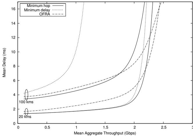
Fig. 4. Mean delay vs. mean aggregate throughput performance of different FiWi routing algorithms for (i) a conventional 20 km range and (ii) a 100 km long-reach wavelength-routing WDM PON and  $B = 100$ .
