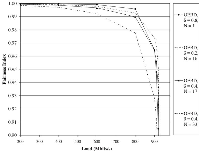
Fig. 6. Excess fairness benchmark,  $f_e$ , for mid-range RTT (up to 10 km).
