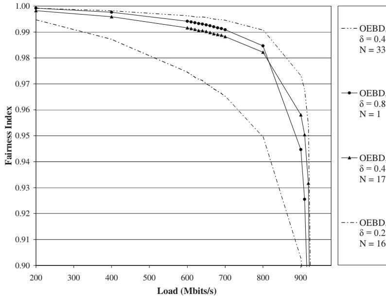
Fig. 7. Excess fairness benchmark,  $f_e$ , for longer-range RTT (up to 100 km).
