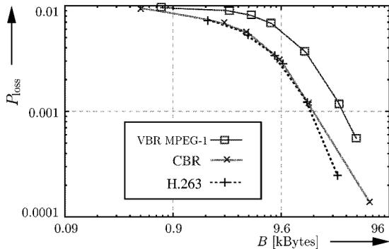
Fig. 9. Client starvation probability  $P_{\text{loss}}$  as a function of the client buffer capacity  $B$  for  $J = 13$  streams of VBR MPEG-1, CBR, and H.263 video.
