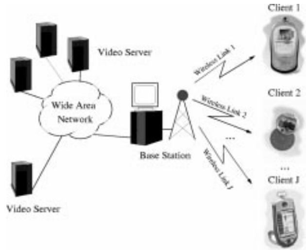
Fig. 1. Architecture: A central base station streams prerecorded continuous media to wireless (and possibly mobile) clients within a wireless cell.
