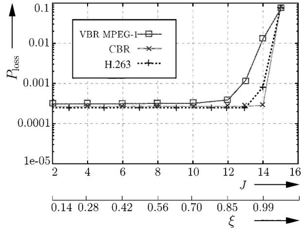
Fig. 8. Client starvation probability  $P_{\text{loss}}$  as a function of the bandwidth efficiency  $\xi$  (obtained by varying the number of clients  $J$ ) for  $B = 32$  kbytes for VBR MPEG-1, CBR, and H.263 video.
