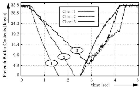
Fig. 3. Sample path plot: Prefetch buffer contents (in kbytes) of 3 clients as a function of time: Client 1 experiences a bad channel.
