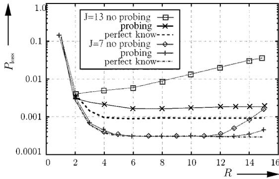
Fig. 5. Client starvation probability  $P_{\text{loss}}$  as a function of the maximum number of channels  $R$  per client for prefetching of VBR video without channel probing, with channel probing, and with perfect knowledge of the channel state.
