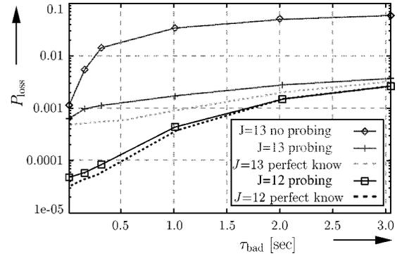
Fig. 4. Client starvation probability  $P_{\text{loss}}$  as a function of the average sojourn time in the “bad” channel state for prefetching of VBR video without channel probing, with channel probing, and with perfect knowledge of the channel state.
