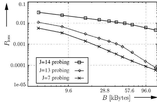
Fig. 7. Client starvation probability  $P_{\text{loss}}$  as a function of the client buffer capacity  $B$  for VBR video.
