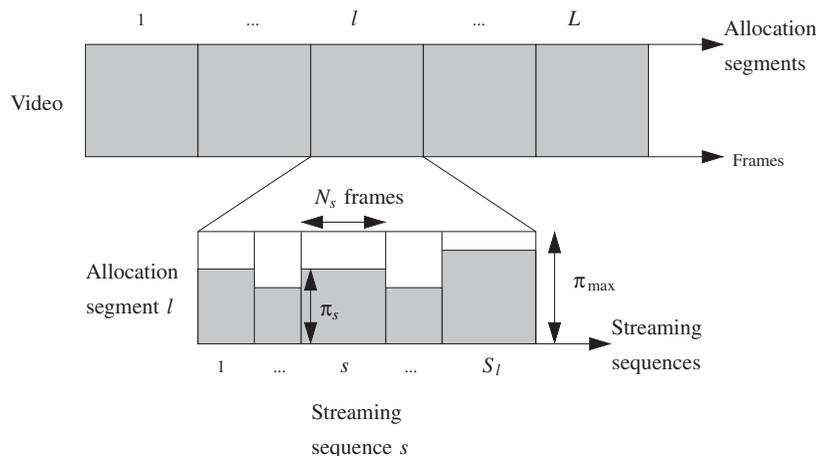
Figure 1. The video is partitioned into  $L$  allocation segments, each consisting of  $S_l$  streaming sequences.
