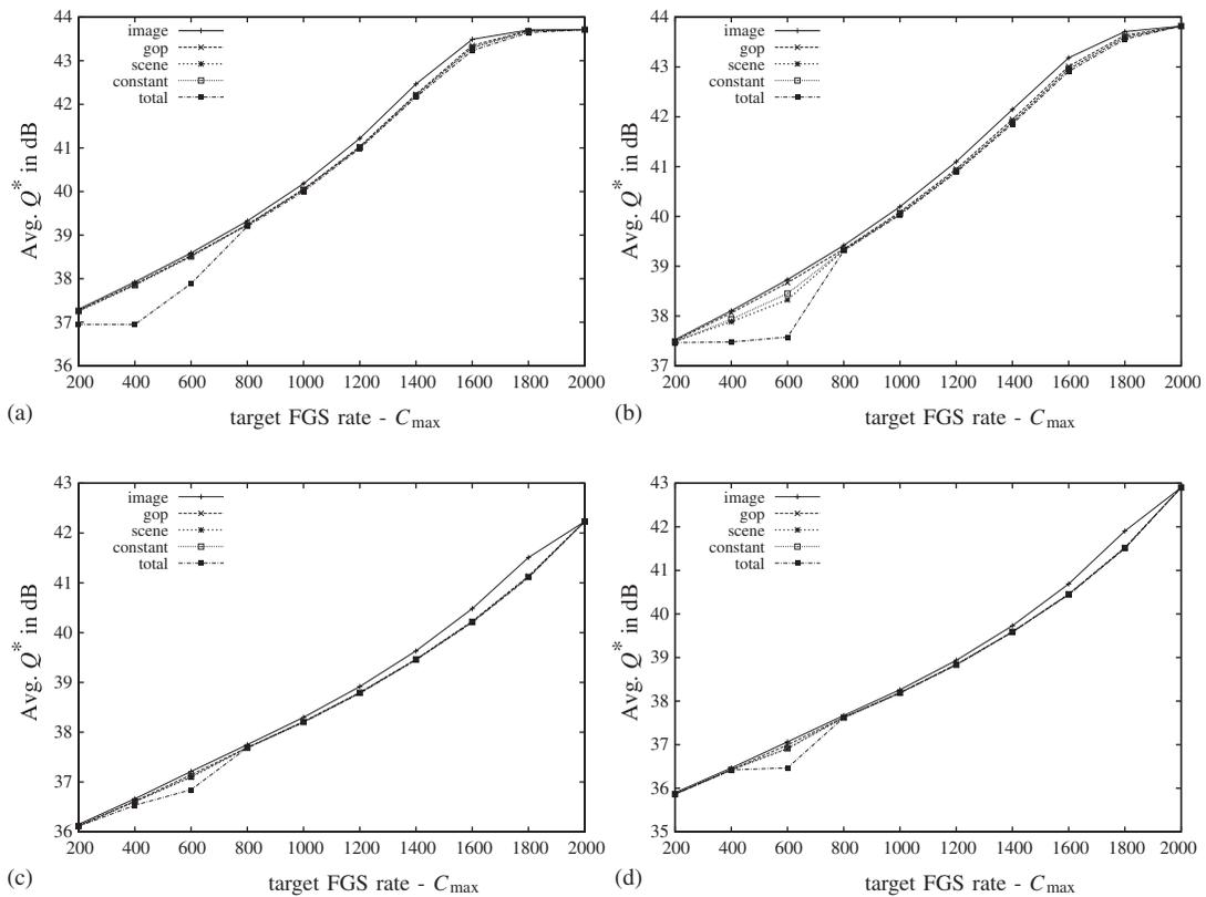
Figure 3. Maximum (PSNR) quality  $Q^*$  averaged over the individual allocation segments as a function of bit rate allocation  $C_{\max}$  in kbps for (a) The Firm, (b) News, (c) Oprah with Commercials, and (d) Oprah.
