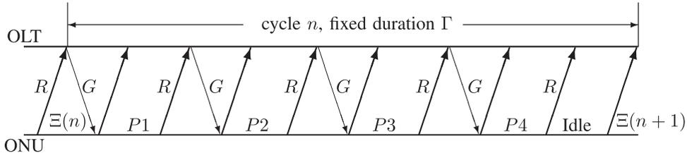
**Fig. 3.** Illustration of low-packet-traffic mode polling: if transmissions from all ONUs in the packet phase P1 following the circuit partition  $\Xi(n)$  reach the OLT more than  $2\tau$  before the end of the cycle, the OLT can launch additional packet polling rounds P2, P3, and P4 to serve newly arrived packet traffic before the next circuit partition  $\Xi(n+1)$ .
