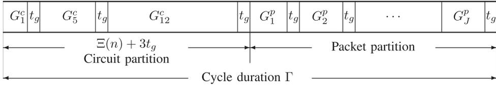
**Fig. 2.** Detailed example illustration of an upstream transmission cycle  $n$ : ONUs 1, 5, and 12 have active circuits with bandwidths resulting in circuit grant durations  $G_1^c$ ,  $G_5^c$ , and  $G_{12}^c$ . Each of the  $J$  ONUs is allocated a packet grant of duration  $G_j^p$  according to the dynamic packet bandwidth allocation based on the reported packet traffic; the packet grant accommodates at least the ONU report (even if there is no payload packet traffic).
