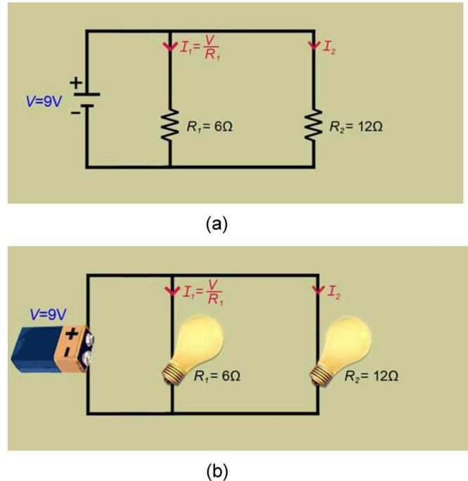
Fig. 1. Sample circuit diagrams from both the no labels (N) conditions: Only the variables denoting the circuit quantities are included in the diagram. There are no text labels that explain the meanings of the symbols for the circuit components in the abstract representation or the illustrations of the circuit components in the contextualized representation. (a) Abstract representation (A). (b) Contextualized representation (C).
