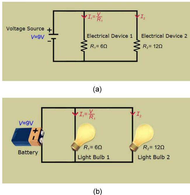
Fig. 2. Sample circuit diagrams from both the static labels (S) conditions: Static text labels explain the meanings of the symbols for the circuit components in the abstract representation or the illustrations of the circuit components in the contextualized representation. (a) Abstract Representation (A). (b) Contextualized representation (C).
