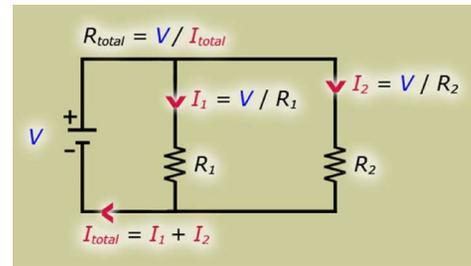
Fig. 1. Sample diagram from the instructional session for the color (C) group. Voltage variables were blue, current variables were red, and resistance variables were black; all variables were black for the black-font (B) group.
