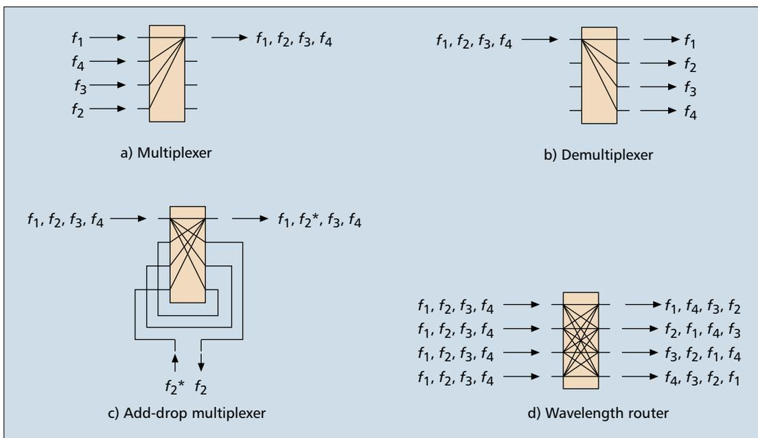
**FIGURE 2.** Basic WDM functions of a  $D \times D$  arrayed waveguide grating (AWG), with  $D = 4$ .
