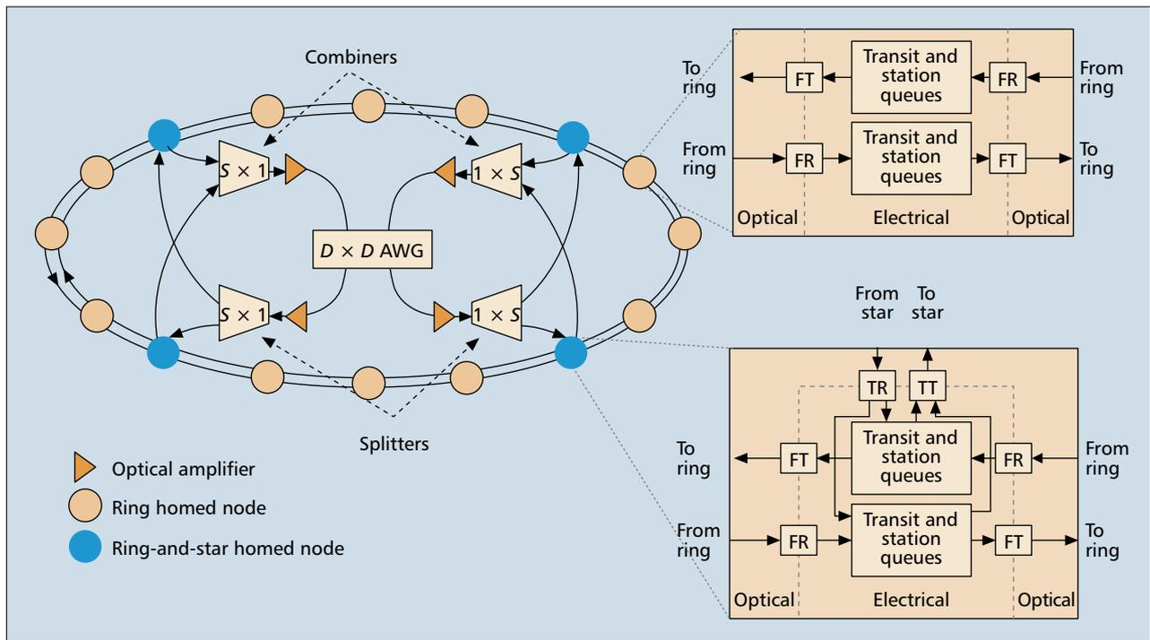
**FIGURE 6.** Hybrid star-ring multihop WDM network: A subset of the ring nodes are interconnected by an AWG based single-hop star WDM subnetwork.
