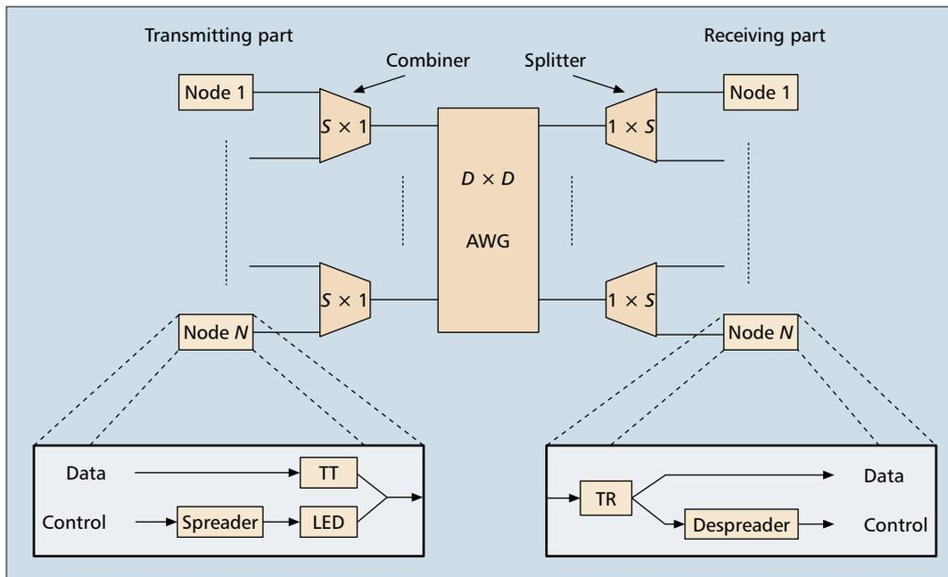
FIGURE 3. Network and node architecture of the TT-TR AWG-based single-hop star WDM network.
