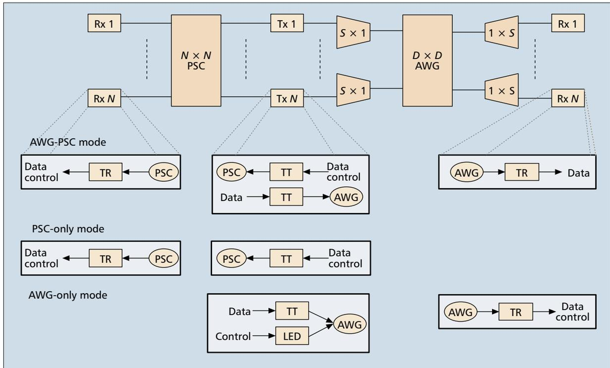
**FIGURE 5.** AWG|PSC single-hop star WDM network: detailed node architecture with transmitter and receiver connections to AWG and PSC for the three different modes of operation, where a given node's transmitter and receiver are collocated. (The AWG and PSC are arranged in parallel; for illustration the network is "unfolded" here.)
