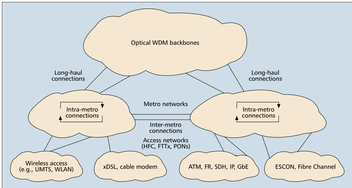
**FIGURE 1.** Network hierarchy: metro networks interconnect access and local networks, which employ a wide variety of networking technologies and provide a range of increasingly higher-speed services, with the high-speed optical WDM backbone networks.
