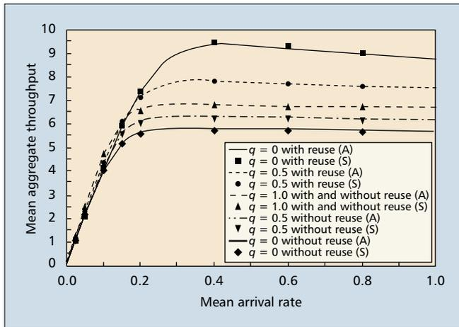
**FIGURE 4.** TT-TR AWG-based single-hop star WDM network: mean aggregate throughput (packets/frame) vs. mean arrival rate (packets/cycle) with and without spatial wavelength reuse for different fractions of long data packets  $q \in \{0, 0.5, 1.0\}$ .
